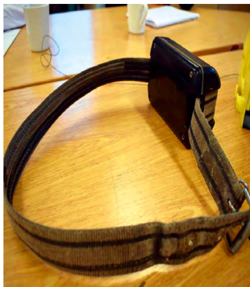
Cow collar with the sensing unit
